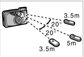
The coverage of the remote controller is up to about 5 m when used directly in front of the camera, and up to about 3.5 m when used at a vertical or horizontal angle of 20°.
